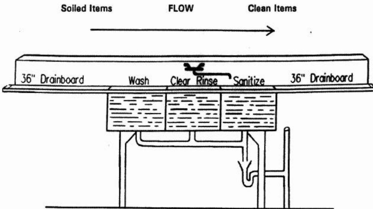
Recommended warewashing arrangement using three-compartment sink. Drainboards for soiled dishes and for cleaned utensils must be adequate. A 36" drainboard should have a pitch of  $\frac{1}{8}$ " to  $\frac{3}{8}$ " per foot toward the sink.
