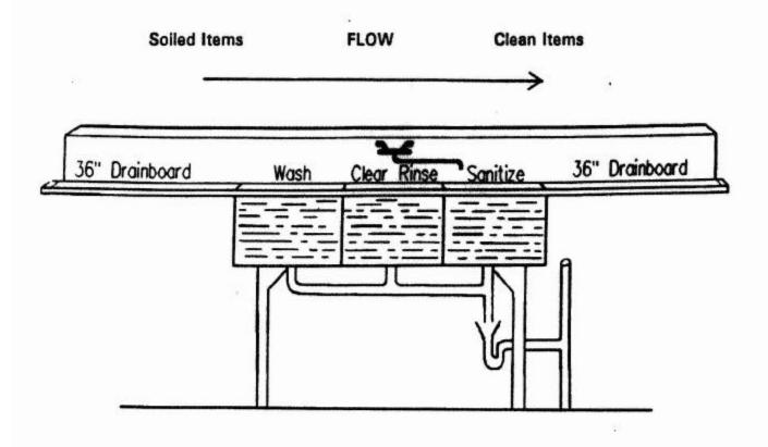
Recommended warewashing arrangement using three-compartment sink. Drainboards for soiled dishes and for cleaned utensils must be adequate. A 36" drainboard should have a pitch of 1/6" to 3/6" per foot toward the sink.
